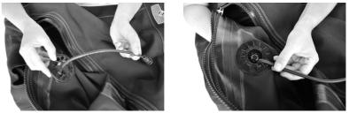
Turn the suit so the inside part is visible and put the connection cable through the nut that will hold the valve. Twist the nut onto the valve until strong resistance, to make sure it will not leak.
