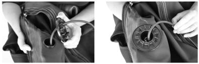
Turn the suit so the inside part is visible and put the connection cable through the nut that will hold the valve. Twist the nut onto the valve until strong resistance, to make sure it will not leak.
