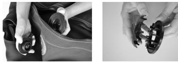
• Prepare all separate parts that are included in the box. Detach your inlet valve and disconnect the cover lid from the valve nut.
